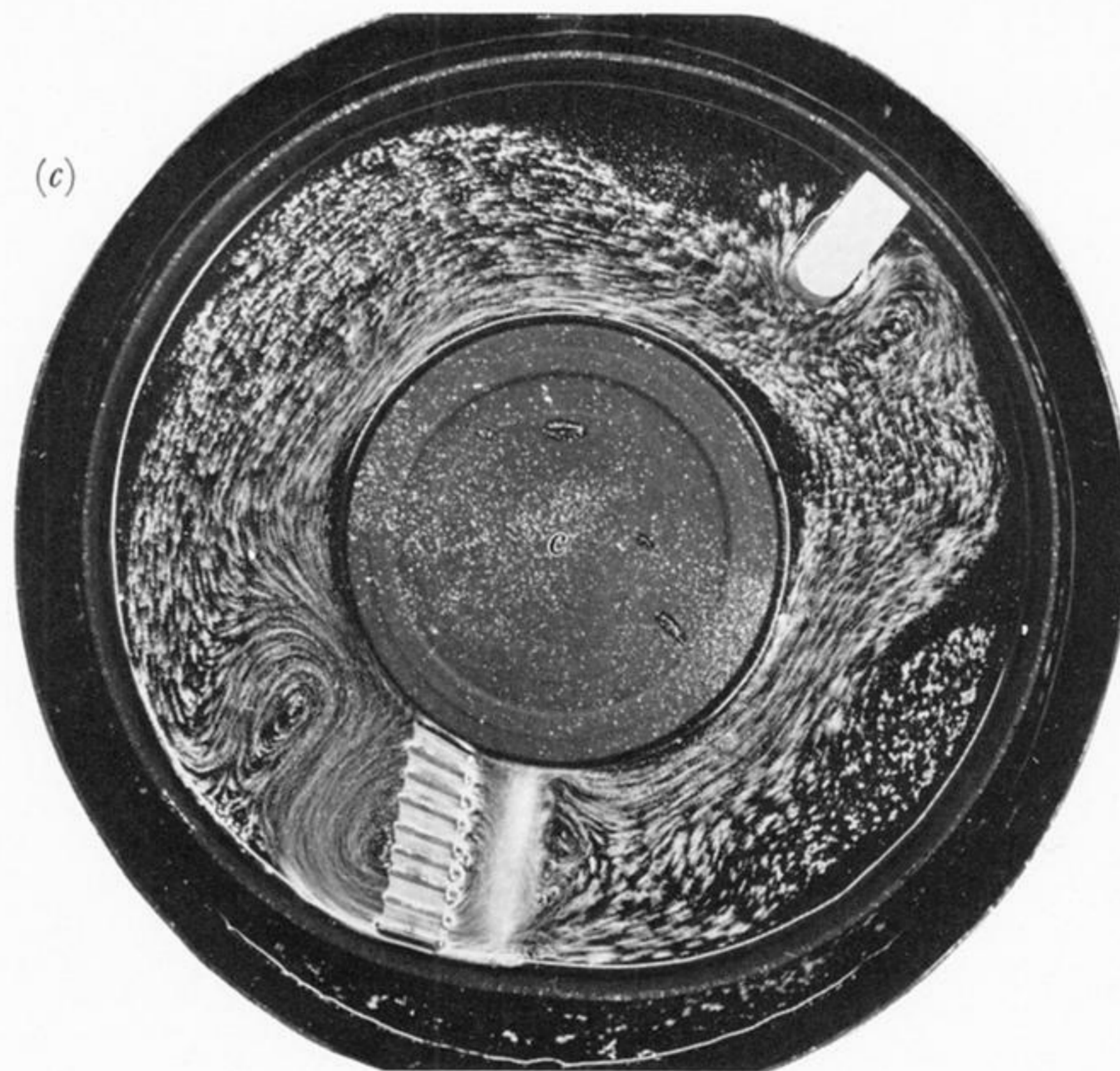
FIGURE 9. Experimental results of J. W. Elder (private communication) showing the effect of variation of \beta on currents through a model Drake Passage, which is at the top right of each picture. A thin layer (about 1 cm) of fluid is driven clockwise by an impeller which is seen (at the bottom of each picture). The \beta effect is provided by the free surface curvature which is produced by the rotation, and increases from (a) to (c). As \beta increases, so does the asymmetry of the motion through the gap, a western boundary current (corresponding to the Falkland current) being well-established in case (c).
